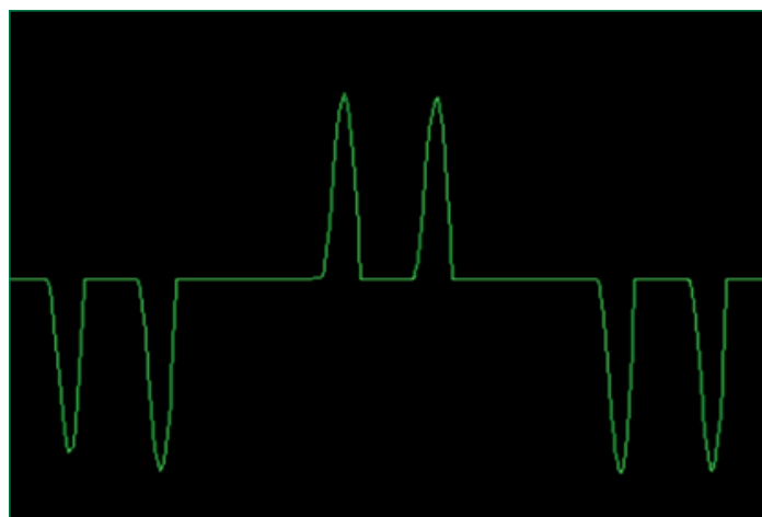
Without Line Reactor
