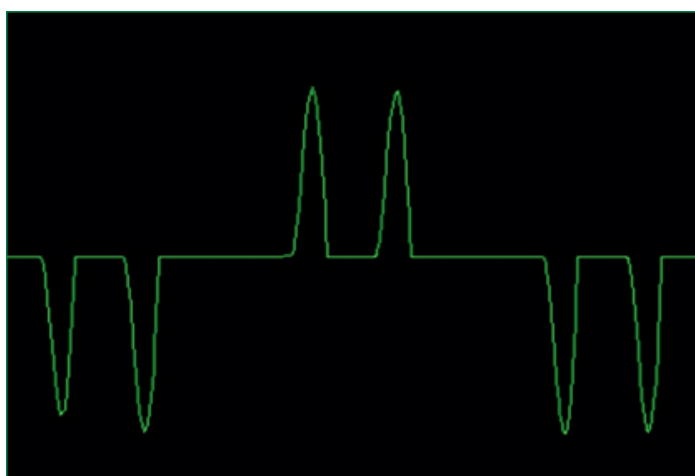
Without Line Reactor
