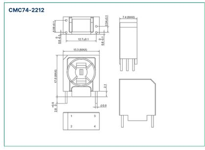
All Dimension in mm; Tolerance According: ISO 2768-m
