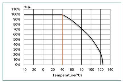
If the ambient temperature exceeds the specified limit, the nominal current needs to be reduced according to the thermal Derating graph shown above.
