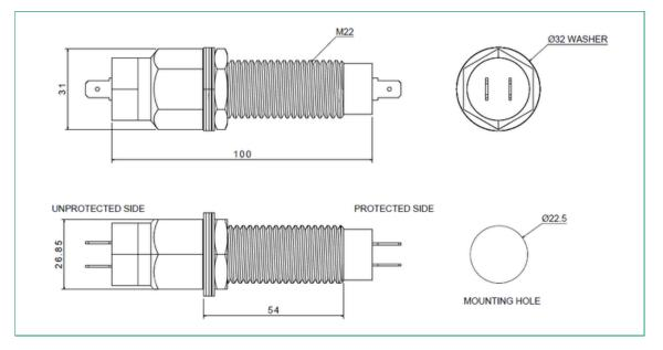
Note: All dimensions in mm; Tolerances according to ISO2768-C
