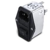
**MF160** 250VAC | 1A to 10A | 50/60Hz IEC Inlet Mounting with Fuse and Switch
